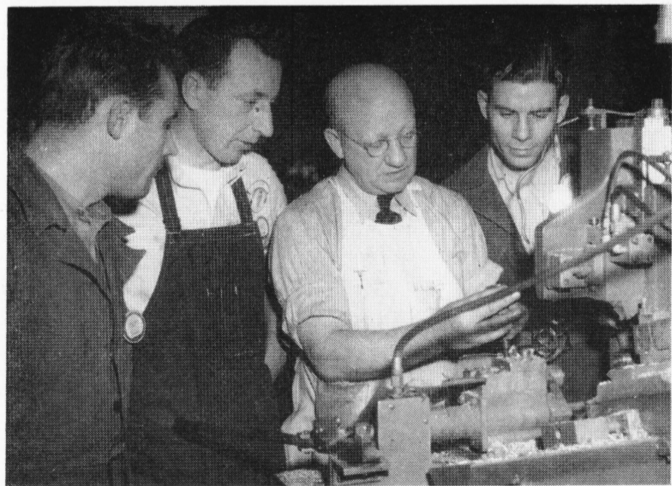
Chucking Toolsetter George Lloyd demonstrates the "this and that" of the low swing lathe used for machining the fuse rings to Bruce Gillett, Jesse Brown and Adam Green. When all these Remington men complete their schooling the Denver Ordnance plant will go into production along very similar lines to the Scovill routine. They will make the major parts, assemble and load the fuses in the new Colorado plant, being the only other plant doing the job nearly as completely as Scovill has been doing it during this and the last world war.
